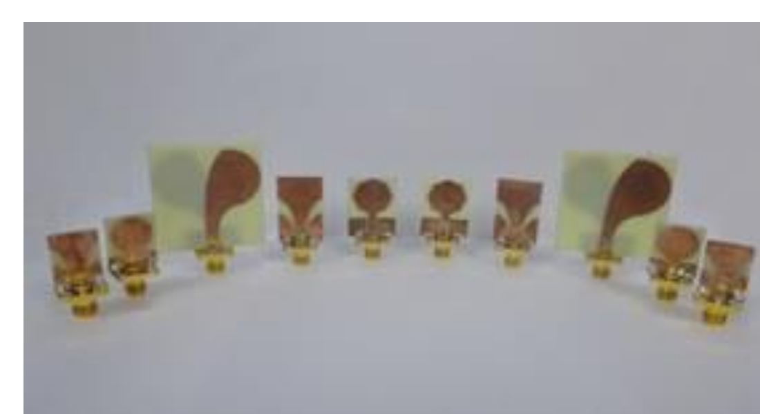
Designed and fabricated miniaturised UWB antennas using GML 60 mil, 3.2 permittivity substrate.
